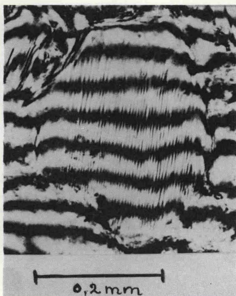
Fig. 8. Non-decorated planar elements in quartz. Two-ray-interference microscope (Leitz).
